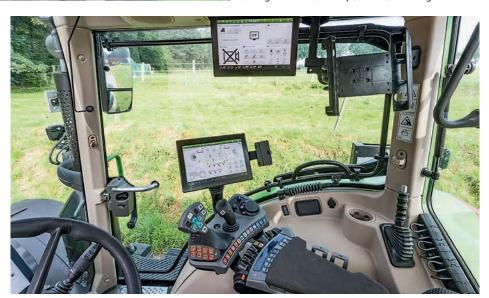
The armrest is completely new on the 724. Also new is the additional display up in the roof, which can be pushed part-way into the roof to improve the to-the-side visibility when on the road.
